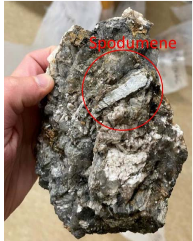
Figure 7: Coarse spodumene (Lithium bearing pyroxene) in rock chip sample from RHW pegmatite
