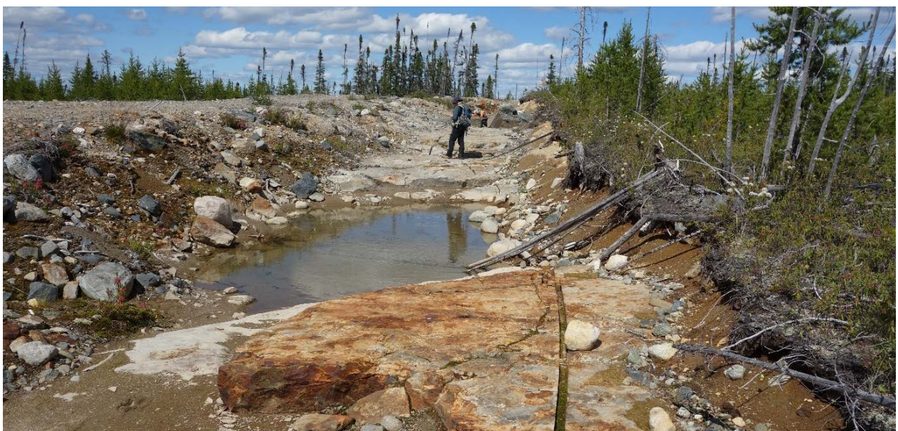
Figure 8: Example of exploration scraping and trenching - Suzanna Trench - Eastmain Gold Project
