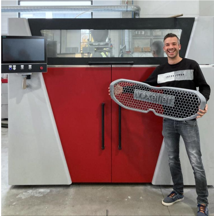
Large parts printed in one piece in PA12 material on new VX1000 HSS printer (in the background)
