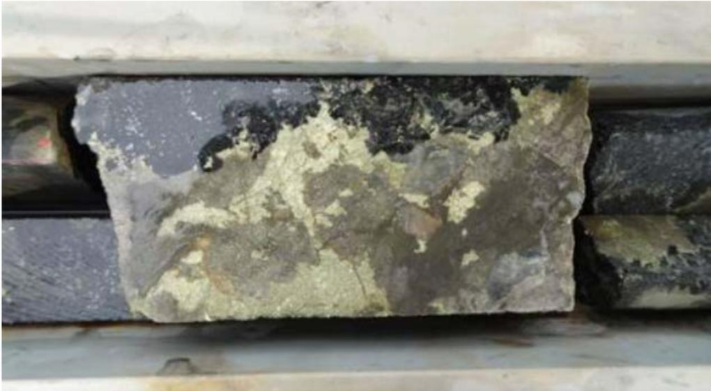
**Photo 4 – Chalcopyrite-Pyrrhotite Mineralisation at 350m depth in drillhole SHDD016**
