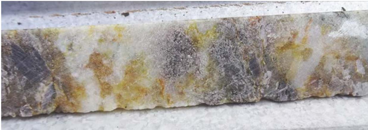
**Photo 8 – Spodumene in drill core from drillhole KSDD001 at Kamativi, Zimbabwe**
