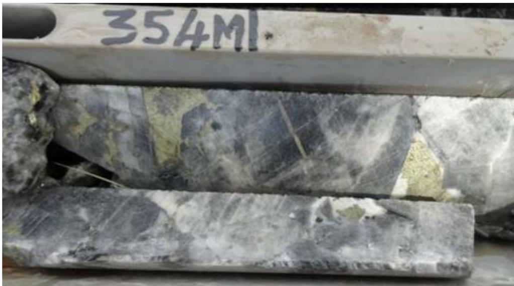
Photo 3 - Chalcopyrite Copper Mineralisation at 354m depth in drillhole SHDD016
