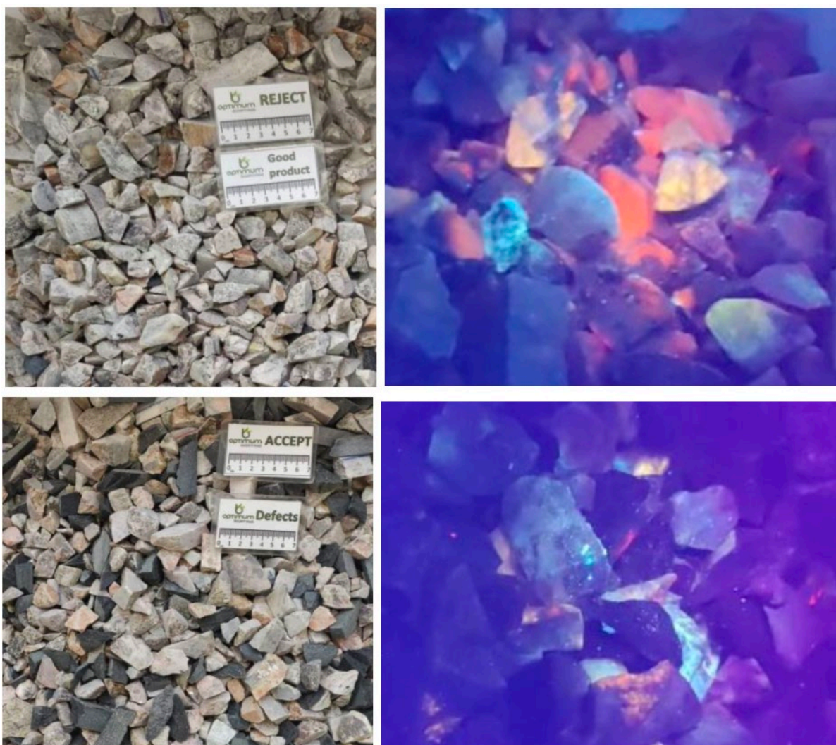
Figure 6 - Dynamic UV ore sorting trial results showing spodumene ore concentrate with its characteristic UV response (top) and waste minerals with no response (bottom).
