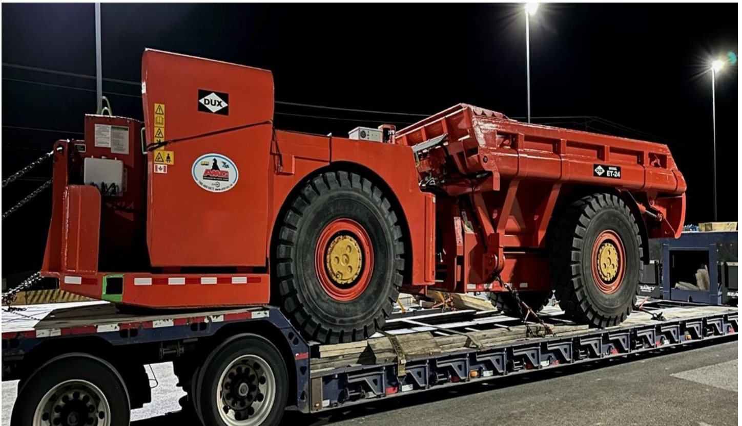
Figure 4 - 20-ton underground haul truck
