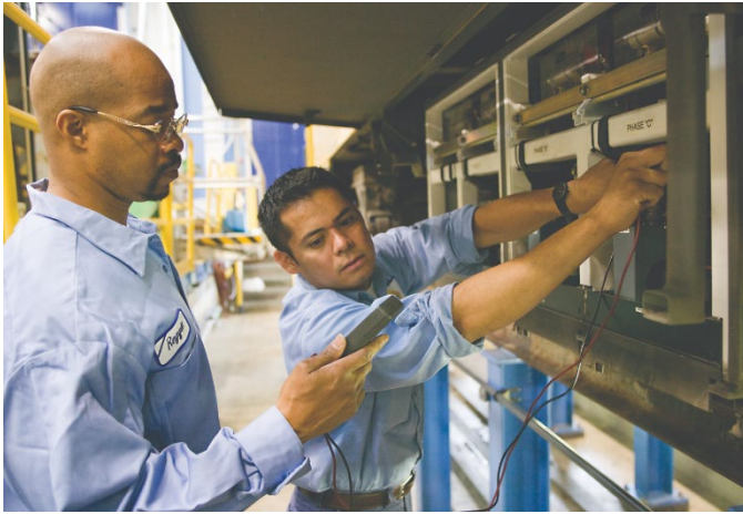
Converting destination signs on light rail vehicles from rollers to digital signs that are easier to update
