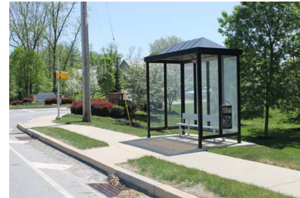
The waiting area typically extends outside of a shelter (if present) to connect with the loading area.
