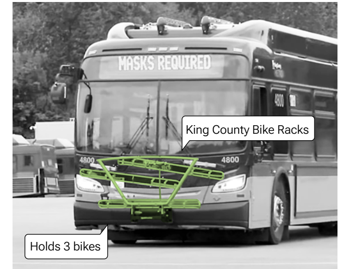
Description: King County Metro bus bike rack that holds 3 bicycles Source: King County Metro
