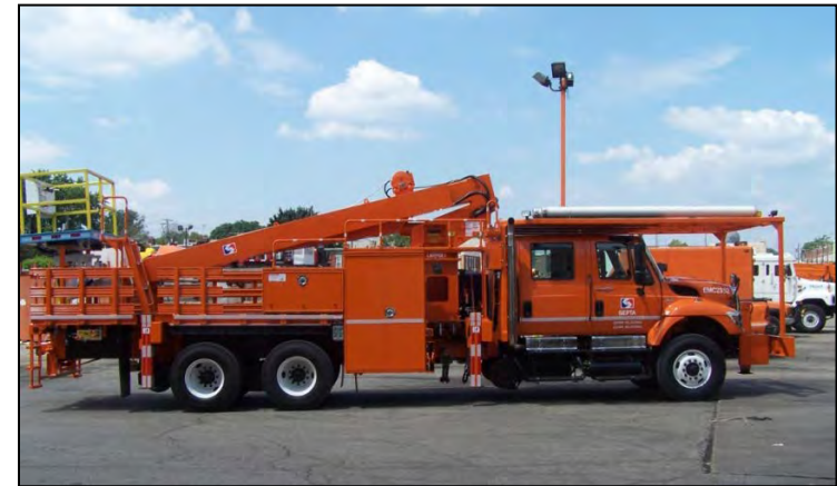
Railroad 6-Person Bucket Truck Supporting Rail Catenary and Signal Programs
