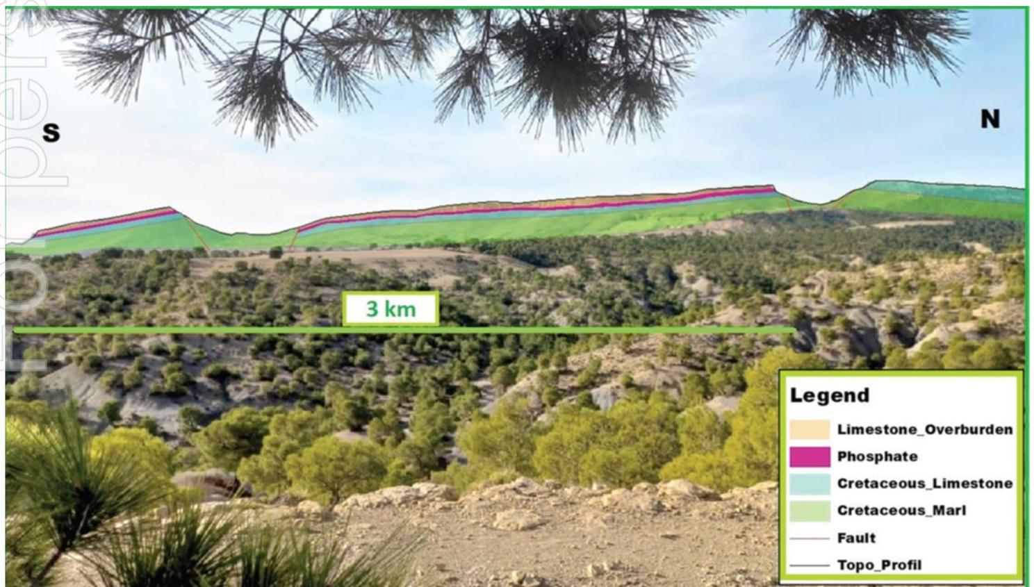
Figure 3 Sekarna Project N \_ S Cross Section A view from the east site
