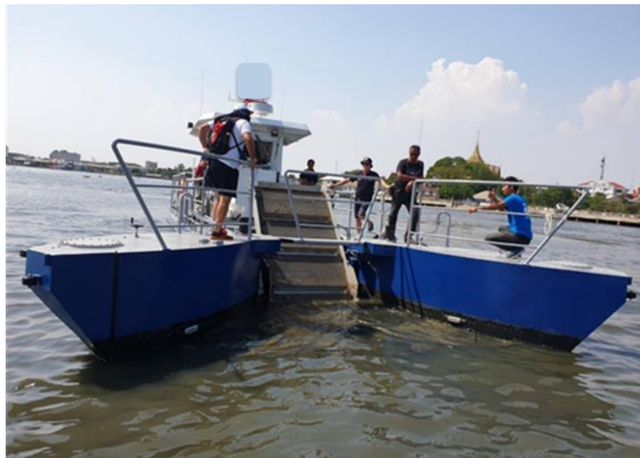
Figure 15. MD collectors of the DMRC – When collecting debris, bow-hull parts be opened to widen the intake area to conveyor
