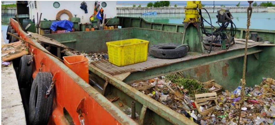
Figure 2. The island-based waste carrier vessel in Indonesia economy, with 120-ton waste capacity. Operation route from Seribu islands to Muara Angke port in Jakarta, Indonesia [6], [12].
