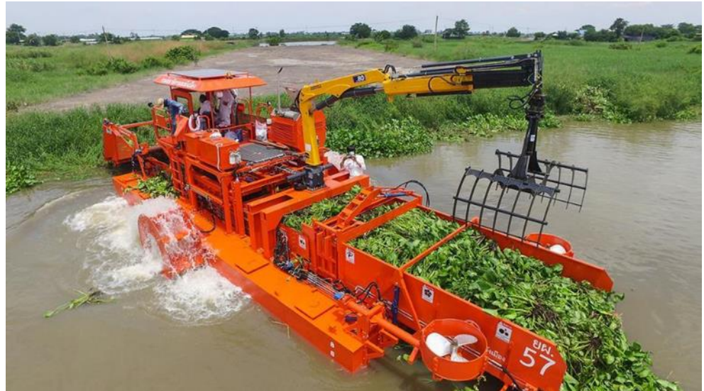
Figure 18. Waste/hyacinth collectors of the Department of Public Works and Town & Economy Planningas
