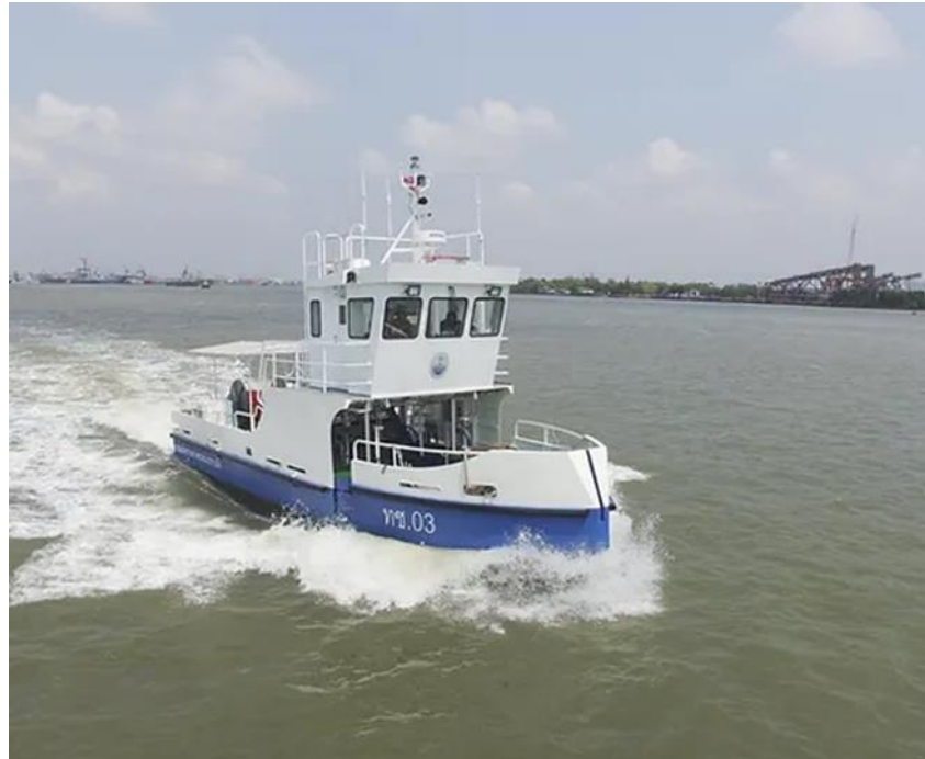
Figure 16. MD collectors of the DMRC – When Sailing, the bow hull closed to minimize drag force
