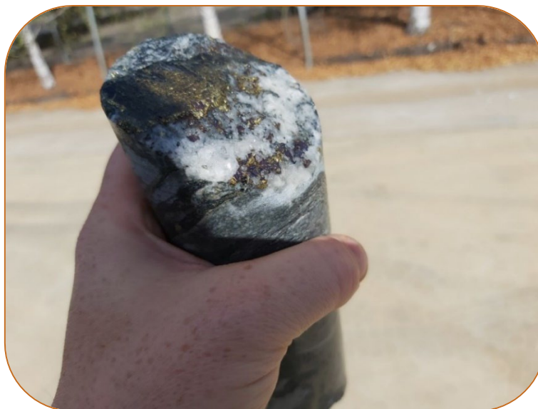
Figure 4: Bornite (Grey-purple) with coarse grained chalcopyrite (brassy) in sugary quartz, 142m - 142.05m (CANDD006)
