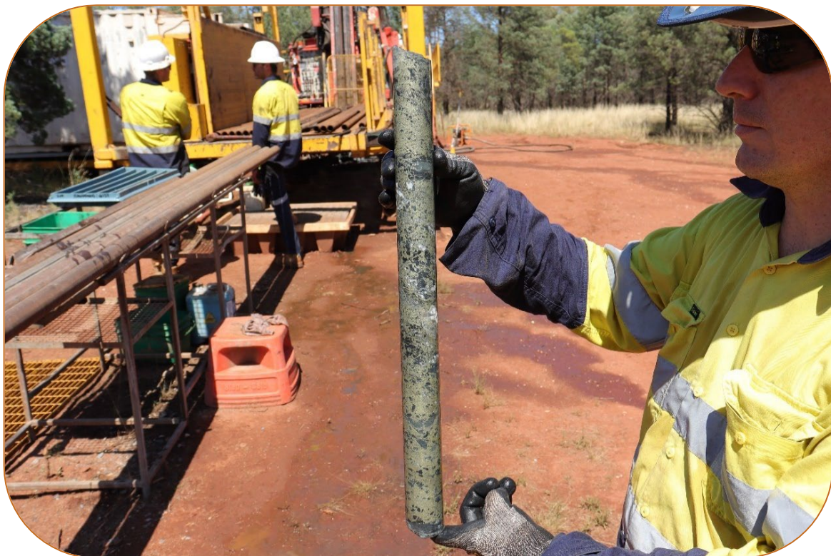
Figure 1 – Massive to semi-massive chalcopryrite intersected from 425.2 metres in CANDD006 1
