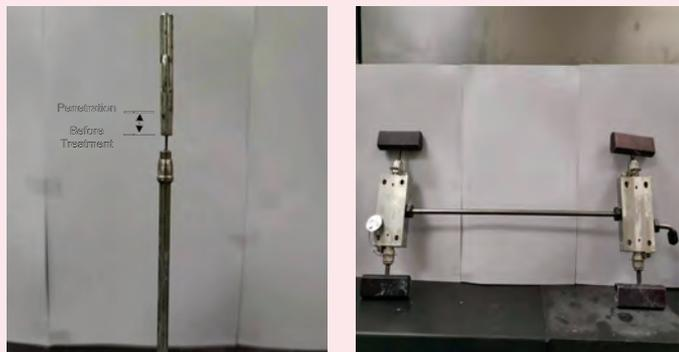
The tube was filled with the chemical shutoff material and placed in the flooding system. Initially, both valves were closed to ensure that the material stays in the tube during the curing time at 200 °F.
