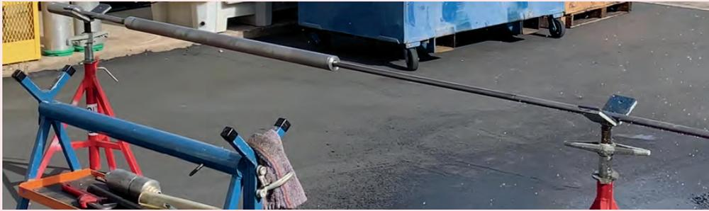
**Fig. 5** The SLT endurance test fixture.
