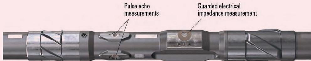
in an OBM environment, was utilized to achieve the well objectives, Fig. 1<sup>1</sup>. The sensors send the pulses through the drilling fluid by the electromagnetic sub-system. These pulses are sent into the formations at a wide range of frequencies to produce the resistivity images of the subsurface geological structures of the formations.
