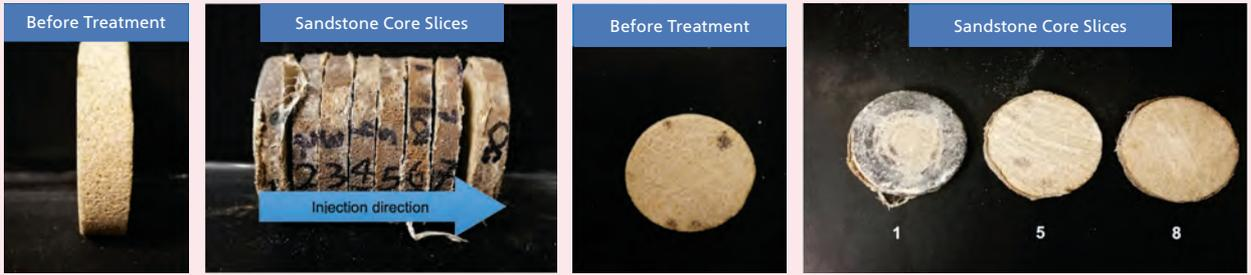
**Fig. 9** Microscopic photos of the sandstone core samples (1, 5, and 8) before treatment and after treatment.
