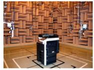
The inside of the acoustic test laboratory
