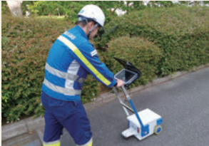
Gas pipes survey using a radar locator
