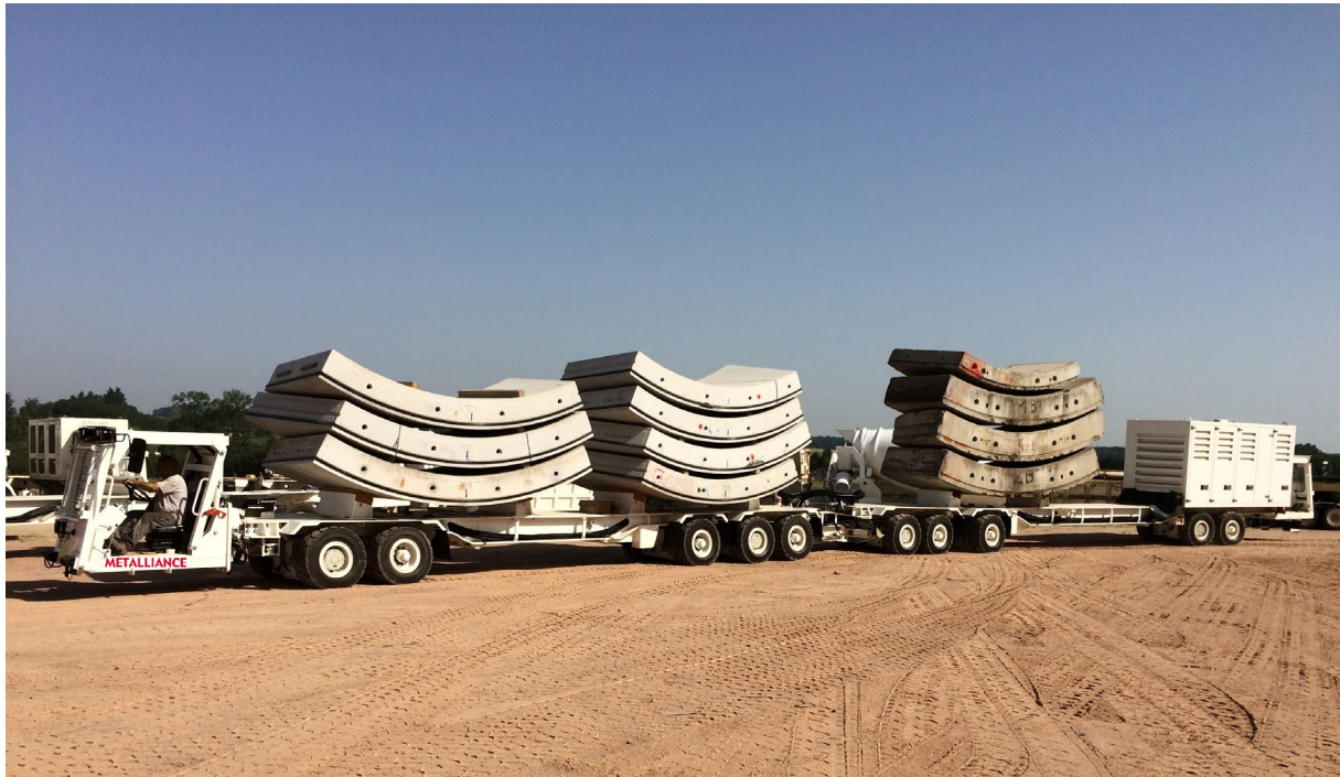
TSP of the METALLIANCE range for transporting segments
