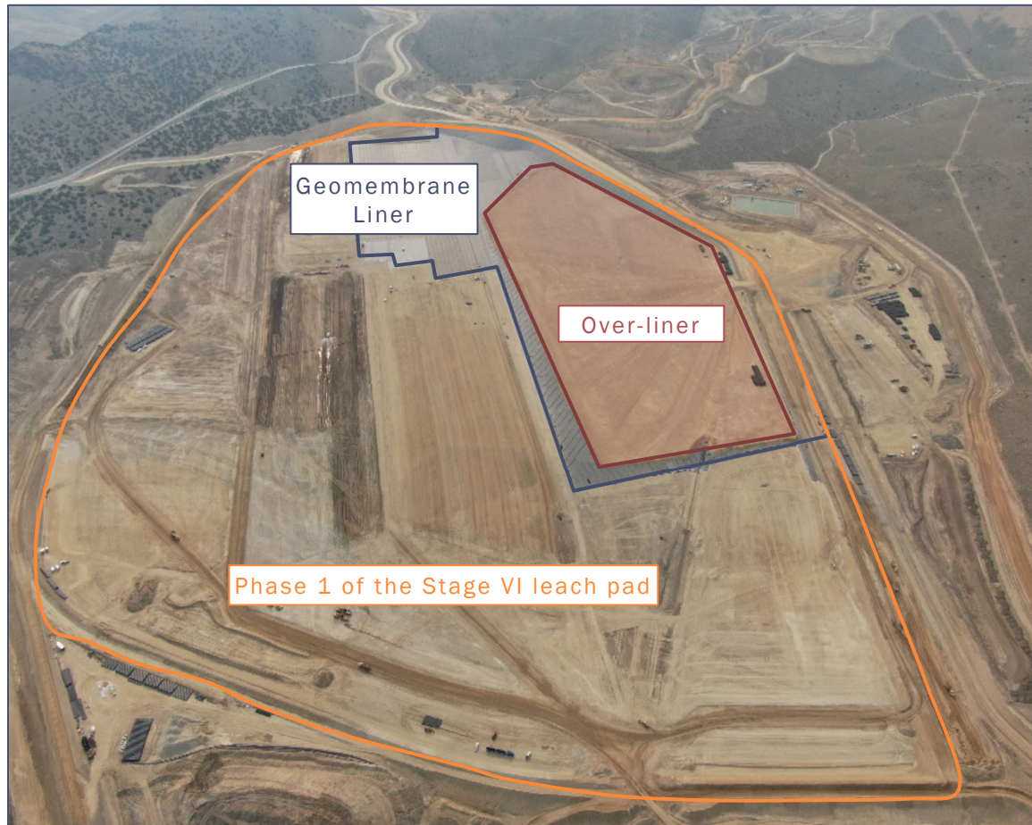
Aerial view of liner being placed on new 300 million ton Stage VI leach pad
