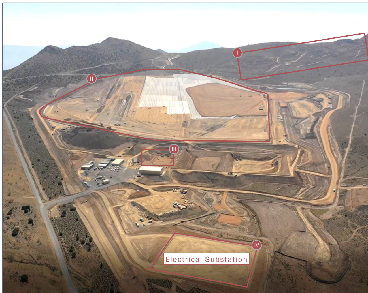
Crushing circuit, including two HPGR units (capacity of ~28.5M tons/year)
