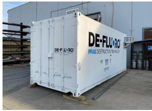
**D**egradation via **E**lectrochemical oxidation of per- and poly**fluoro**alkyl substances
