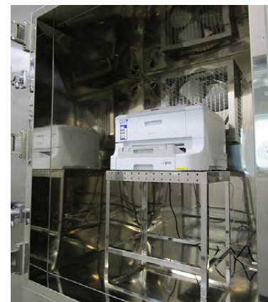
Measurement of substances released by products
