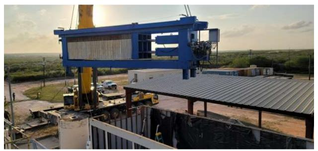
Above: The yellowcake filter press is placed at the Rosita Central Processing Plant, completing the uranium processing circuit.
