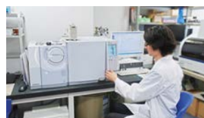
Using gas chromatography-mass spectrometry equipment, inspections are conducted to determine the presence or absence of regulated chemical substances that have the potential to harm the human body.
