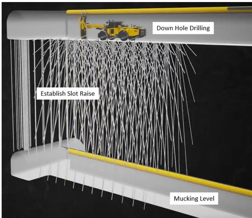
**Figure 16-8 Cross Section View of Longhole Open Stopping**
