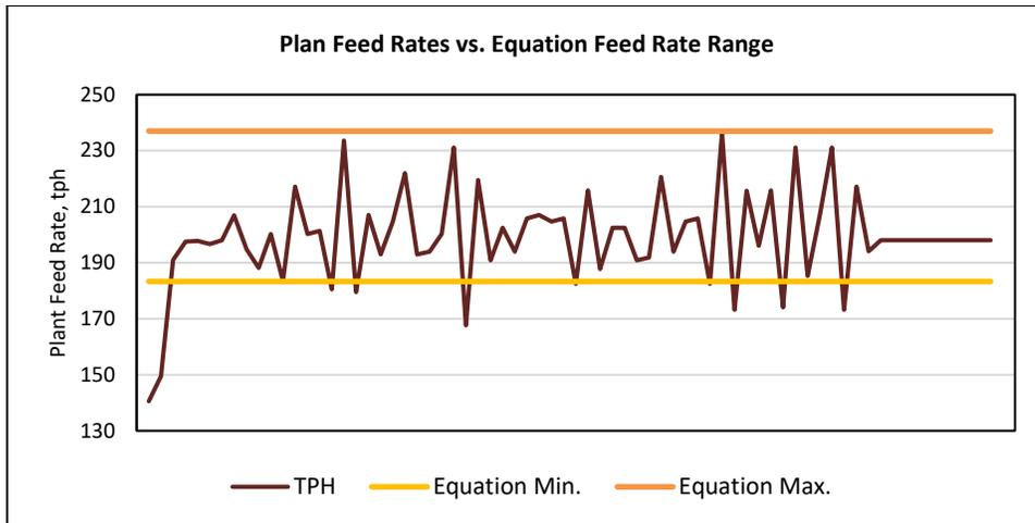
**Figure 13-7 Plan feed rates compared to recovery equation feed rates**
