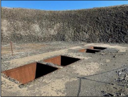
**Figure 17-10 Stockpile feeders (Lain photo)**
