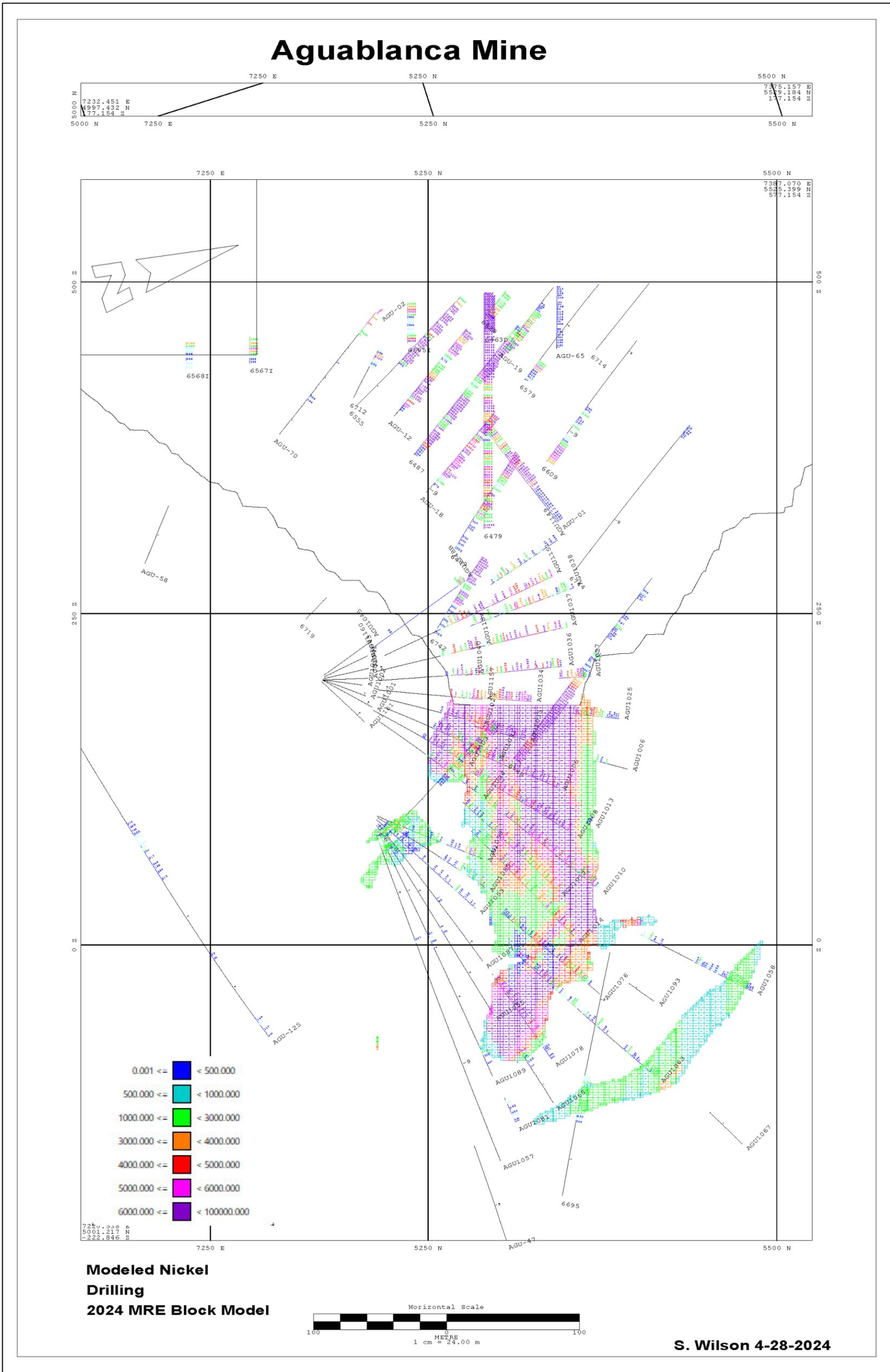
Figure 14-14: Cross Section through the main Aguablanca deposit demonstrating consistency between drilling assay results and the interpolate mineralization for the deposit.
