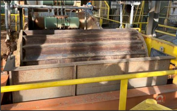
**Figure 17-17 SAG mill discharge rotary magnet**
