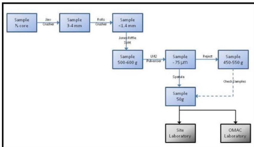
Figure 11-6: Sample preparation flow sheet as used for Aguablanca resource definition samples
