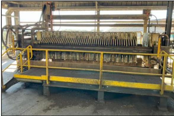
Figure 17-26 Plate and frame filter press
