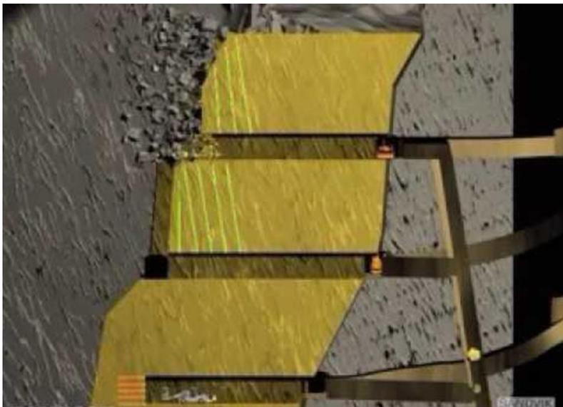
Figure 16-7 Section View of Up Hole Stope Extraction
