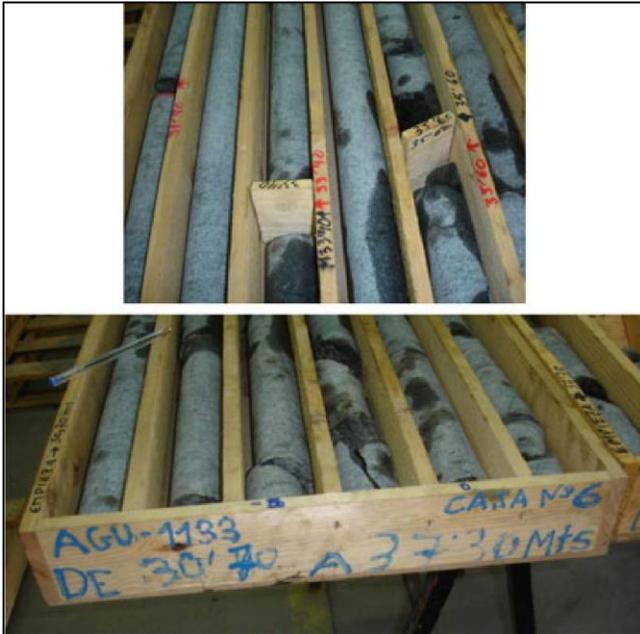
Figure 11-1: Labelling of core boxes for Aguablanca resource drilling
