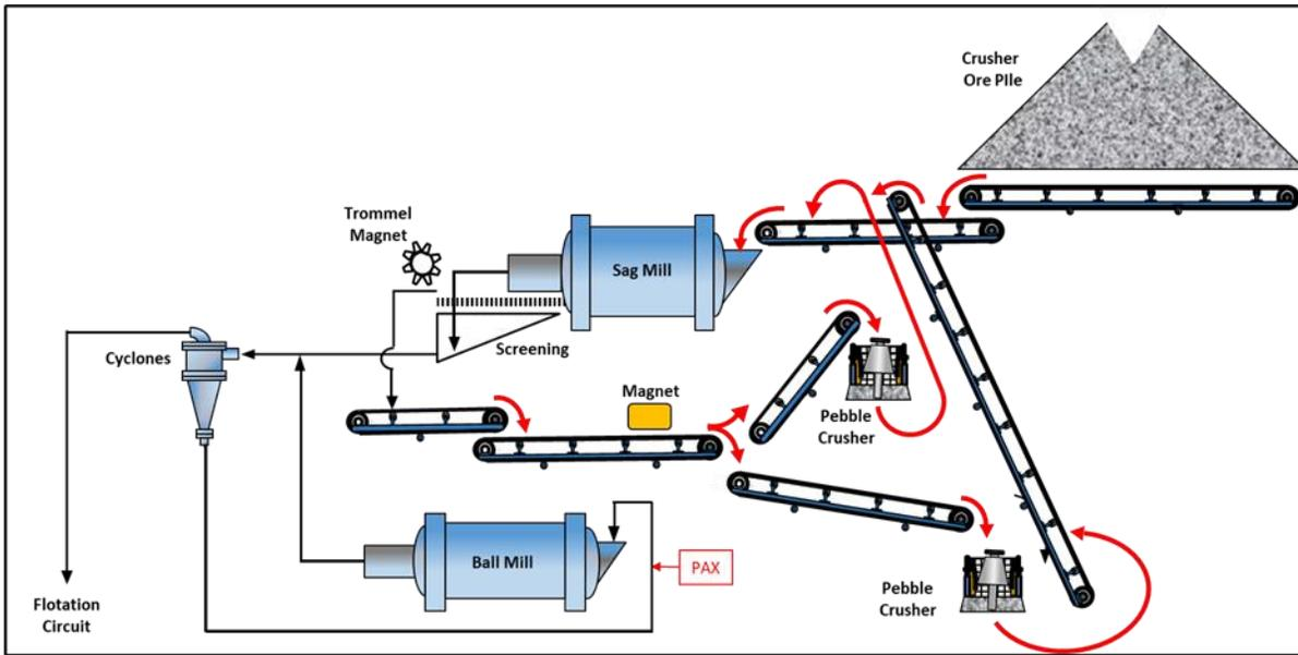
Figure 17-15 Grind circuit flowsheet
