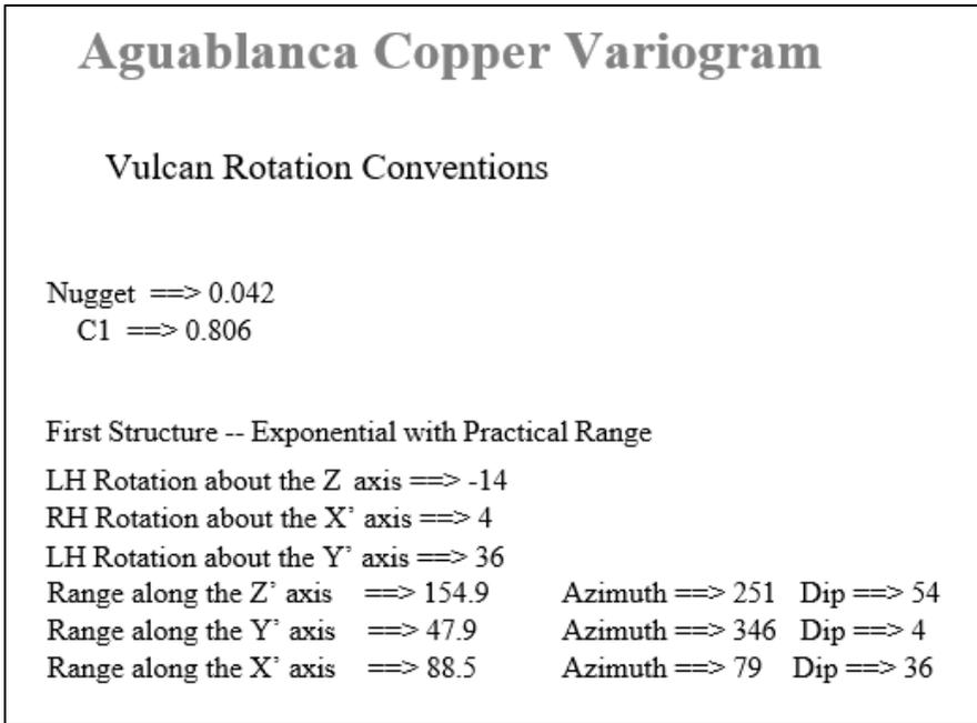
Figure 14-12 Sage2000 copper anisotropy search parameters
