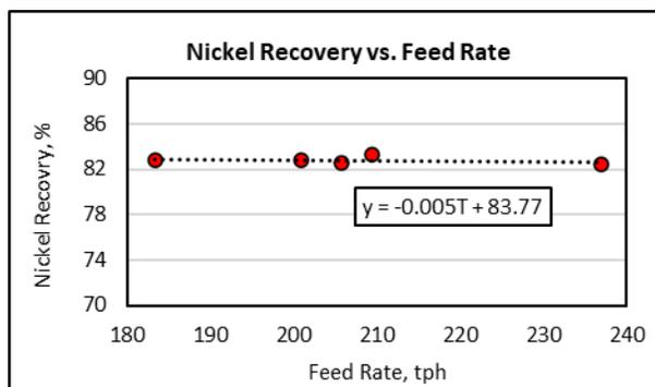
Figure 13-2 Actual nickel recovery vs. feed rate
