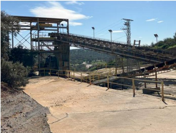
Figure 17-7 Secondary crusher feed conveyor
