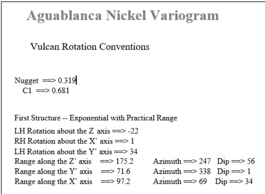
Figure 14-9 Sage2000 nickel anisotropy search parameters
