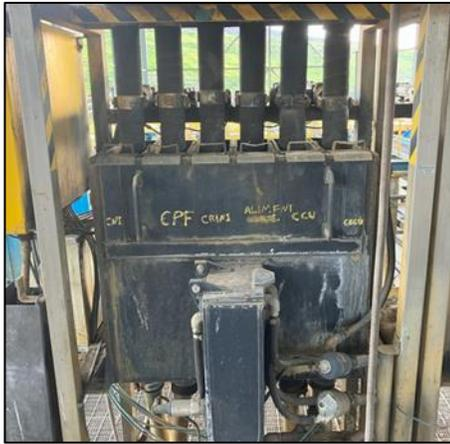
Figure 17-21 On line automated sampler
