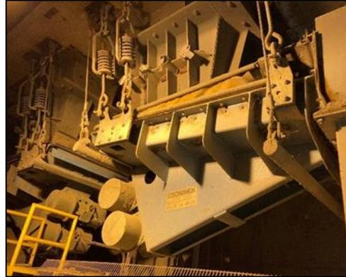
**Figure 17-11 Stockpile feeders (Lain photo)**
