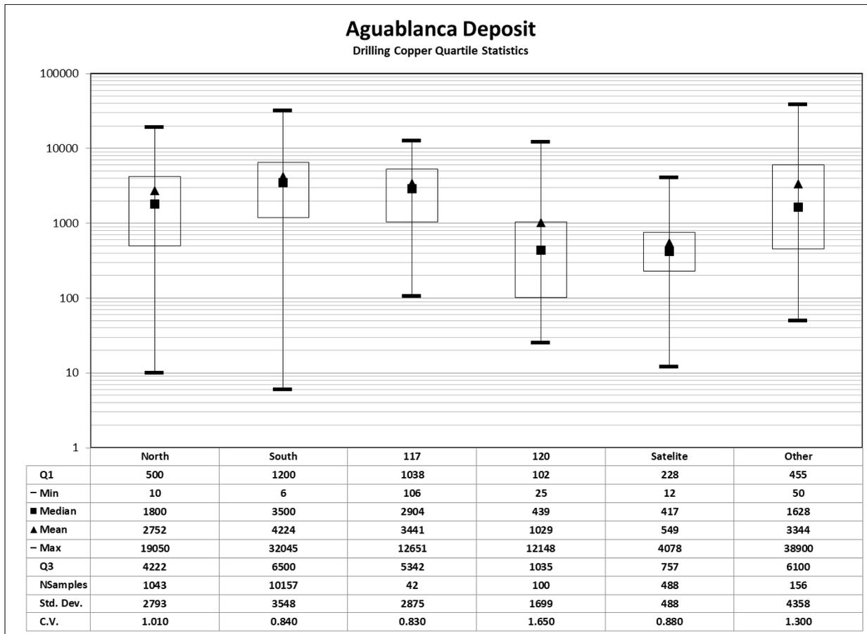
**Figure 14-2 Uncapped copper grade distribution by mineral body**
