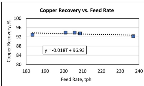
**Figure 13-4 Actual copper recovery vs. feed rate**
