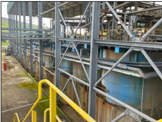
**Figure 17-24 Nickel rougher and scavenger banks**
