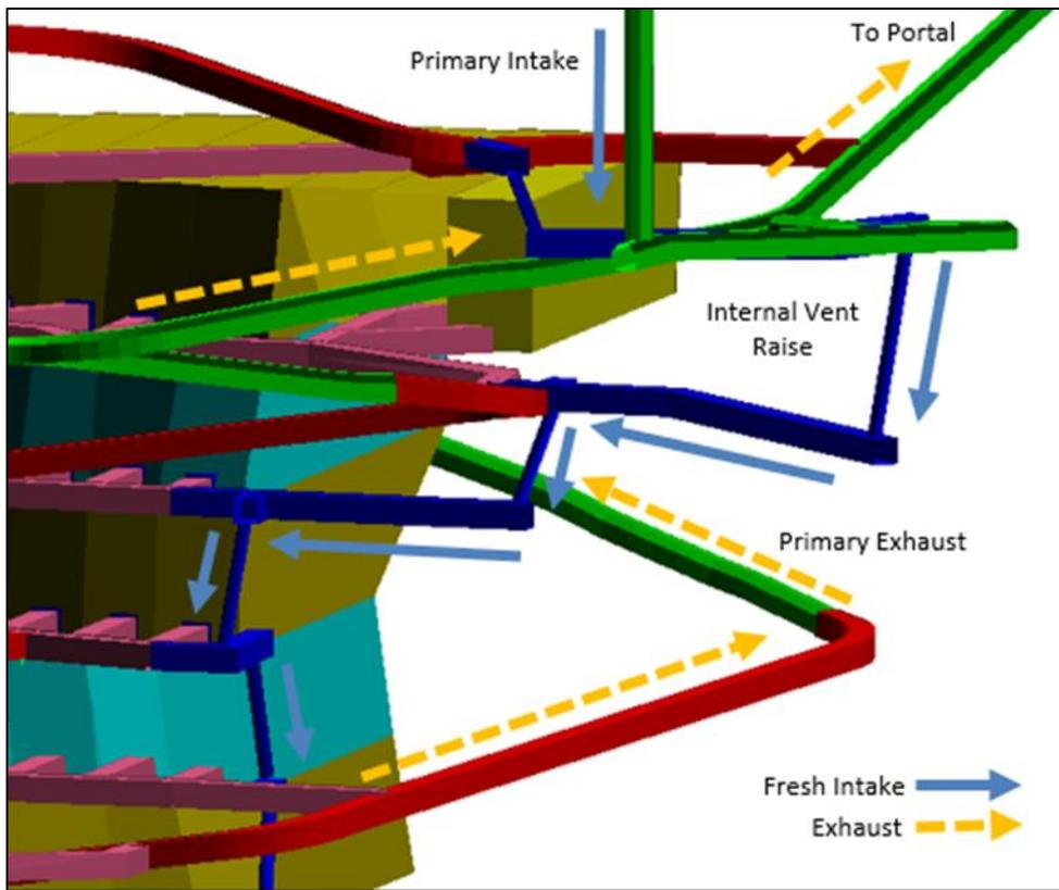
**Figure 16-12 Typical Conceptual Ventilation System**
