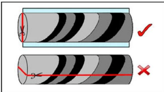
**Figure 11-4: Correct core sawing orientation being used at Aguablanca**
