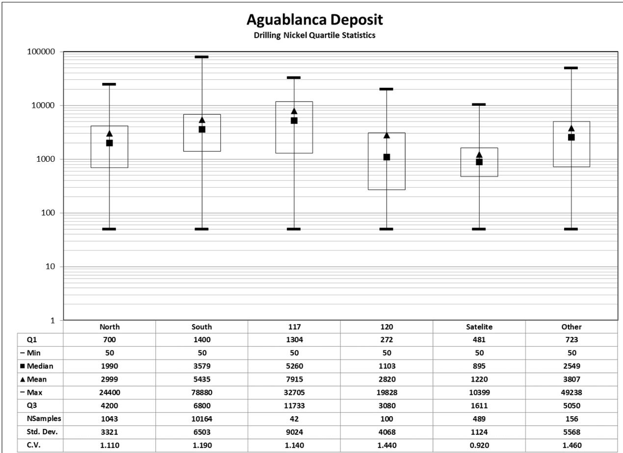
Figure 14-1 Uncapped nickel grade distribution by mineral body
