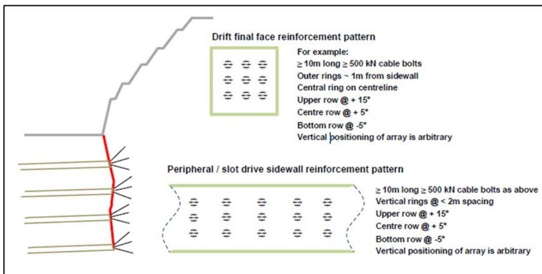
**Figure 16-9 USE Panel Reinforcement Concept**
