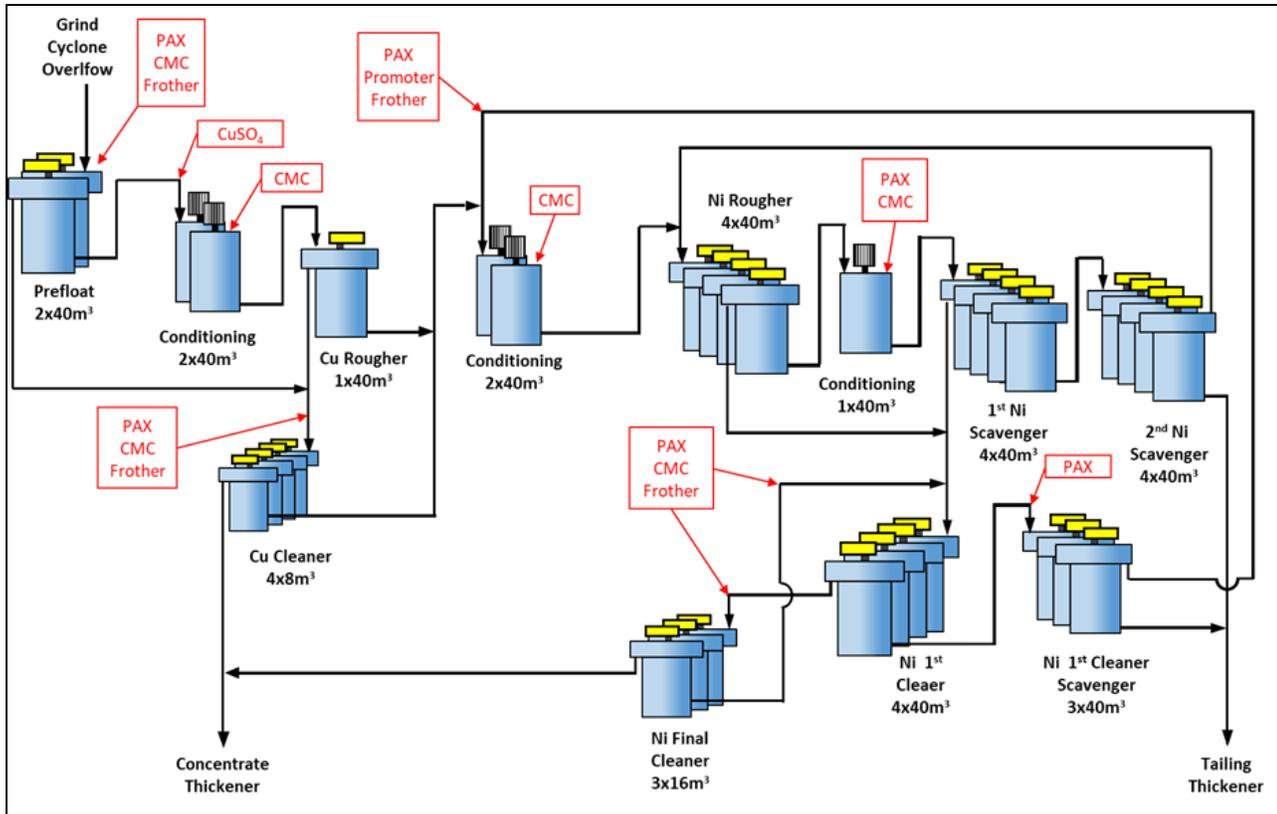
Figure 17-20 Flotation circuit
