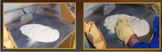
**Figure 11-8: Splitting of pulverized samples using a spatula**
