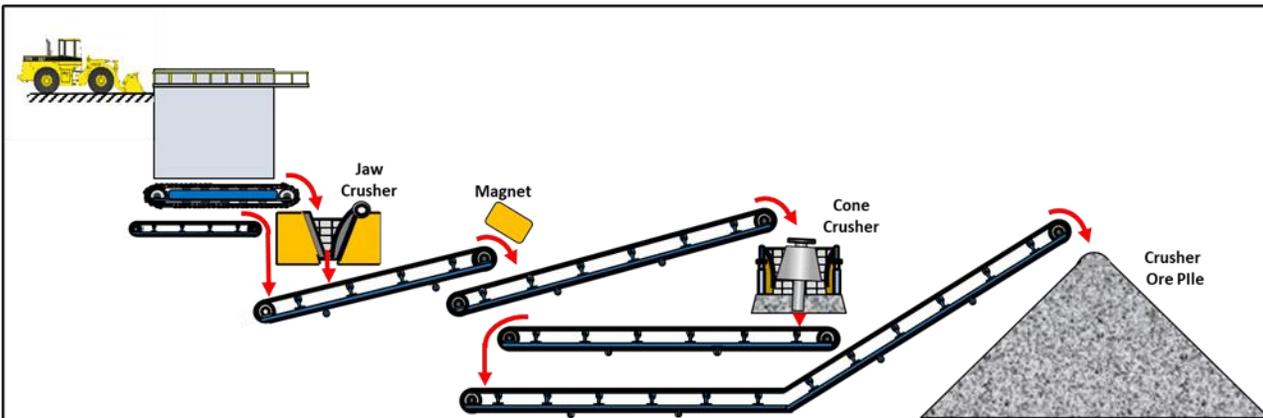
Figure 17-9 Aguablanca crushing circuit
