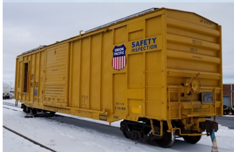
Custom-developed boxcars aid track inspection.
