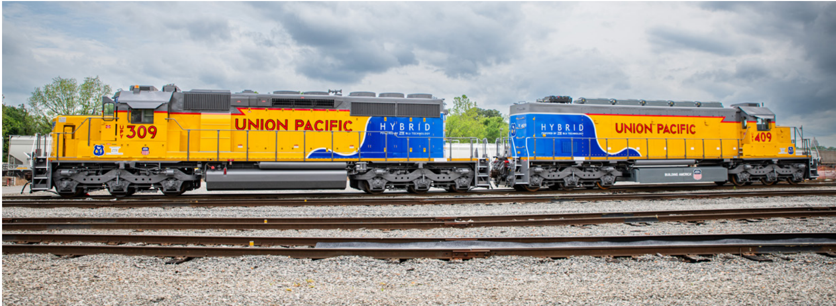
The first of six cutting-edge hybrid battery-electric locomotives designed and built by Union Pacific and ZTR will undergo extensive testing in May 2024.
