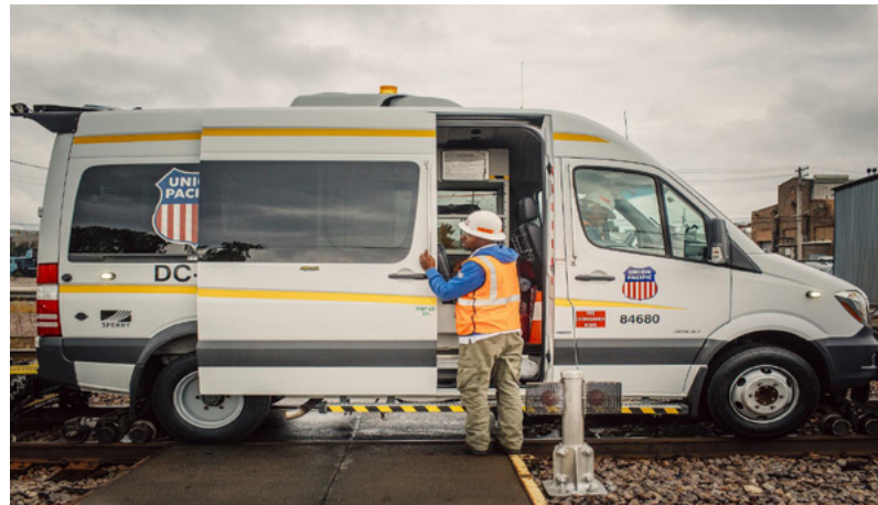
Our DC-56 ultrasonic rail inspection vehicle is used to identify potential rail defects with high frequency sound.
