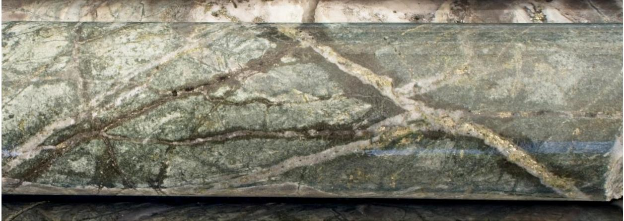
**Image 2.** ELID023, 397.5 m from a 2 m long sample interval reporting **1.07% Cu, 0.003% Mo, 14.6 g/t Ag**. Quartz vein containing a chalcopyrite assemblage in potassic-altered feldspathic arenite. Chalcopyrite is disseminated in the quartz vein and wall rock and in chalcopyrite-pyrite veinlets that overprint the quartz vein. Molybdenite is unusually low in this part of the drill hole. Core is HQ diameter (63.5 mm).
