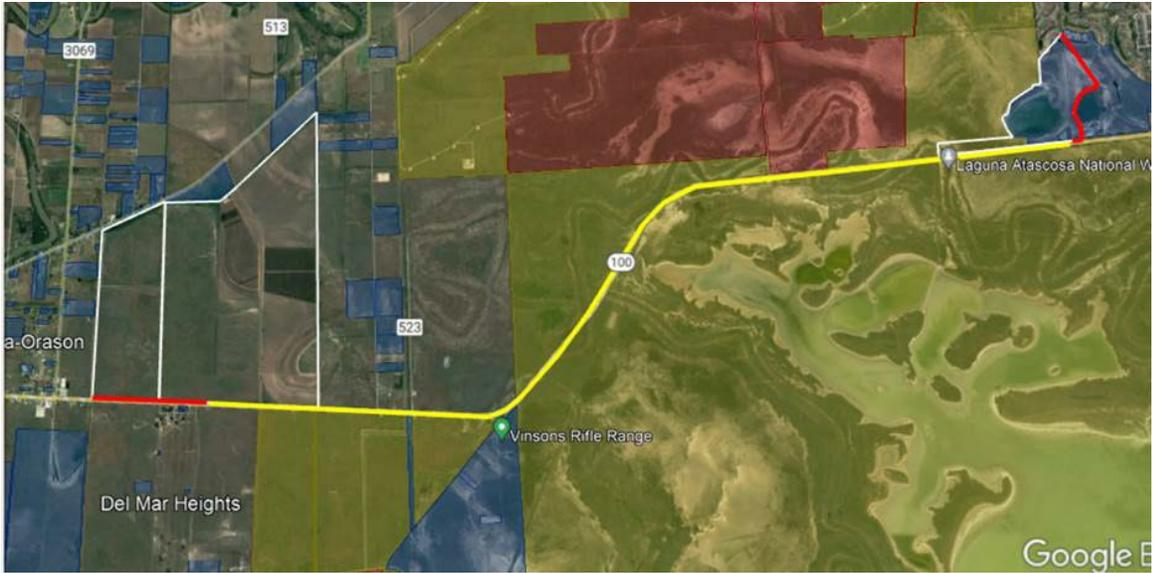
Figure 3. Map of existing fence (yellow line) along SH 100 and proposed fencing extensions (red lines) at Laguna Vista gap and Los Fresnos gap, Cameron County.
