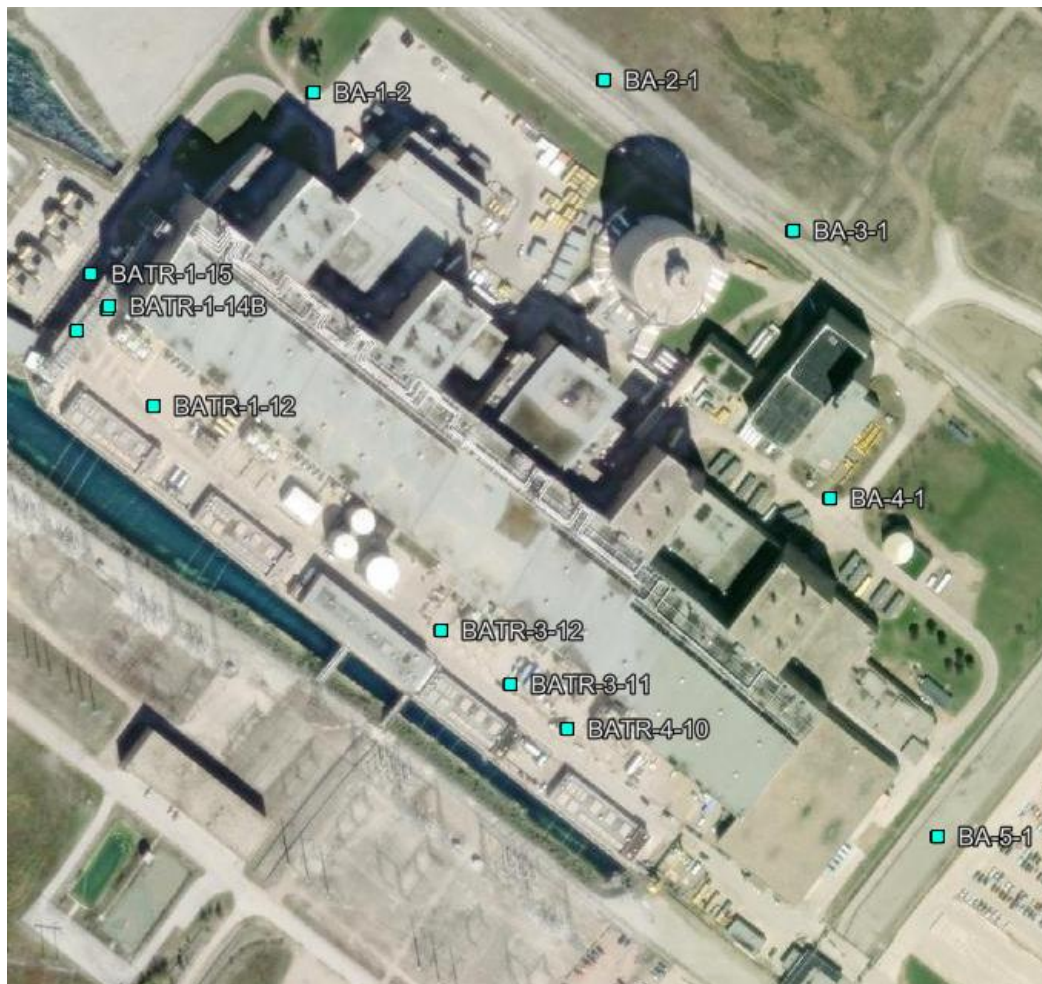
Figure 59 - Bruce A Radiological Groundwater Sampling Locations
