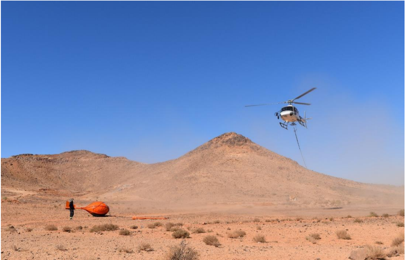
Figure 6 - Preparations for the MobileMt Airborne Geophysical Survey on Boumadine.
